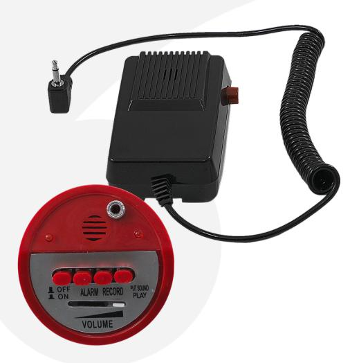
When inserting batteries please take care to ensure correct polarity. Insert the batteries with the (-) marks on the batteries aligned close to the spring in the back cover. When the megaphone will not be used for long periods always remove the batteries to prevent leakage. Please note that using drained batteries will lower the output level.
