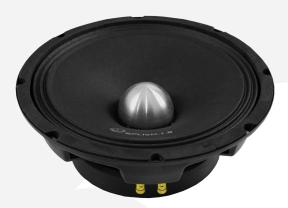
During installation of your SPL10M.1 we recommend that you have music playing as you tighten the speaker into the enclosure or panel. This will allow you to listen and make sure that the basket is not distorted during installation which can result in voice coil rub. It is absolutely essential that the mounting surface for SPL10M.1 is ABSOLUTELY FLAT.
