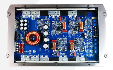
Time to lay on some power. Connect the earth first, then 12V power, then remote. Then connect in the RCA cables and you can move onto setting up sound controls on the amplifier. This description covers the principles of operation – for specific instructions refer to the set up notes for the exact model you are working with.
