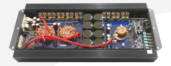
Time to lay on some power. Connect the earth first, then 12V power, then remote. Then connect in the RCA cables and you can move onto setting up sound controls on the amplifier. This description covers the principles of operation – for specific instructions refer to the set up notes for the exact model you are working with.
