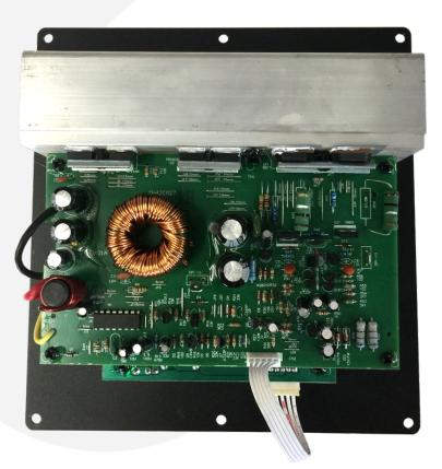
Either fit female crimp terminals to the wires on the bass box or strip back and solder directly to the circuit board. The RED cable is the positive and should be connected to the + terminal.
