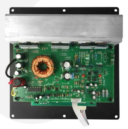
Either fit female crimp terminals to the wires on the bass box or strip back and solder directly to the circuit board. The RED cable is the positive and should be connected to the + terminal.
