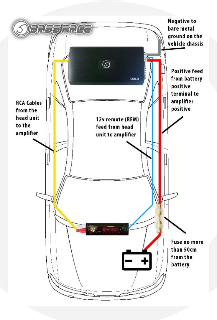
Begin by disconnecting the car battery, taking note of any required precautions suggested by the vehicle manufacturer such as alarm or radio codes, or on board computer or AGM battery requirements.
