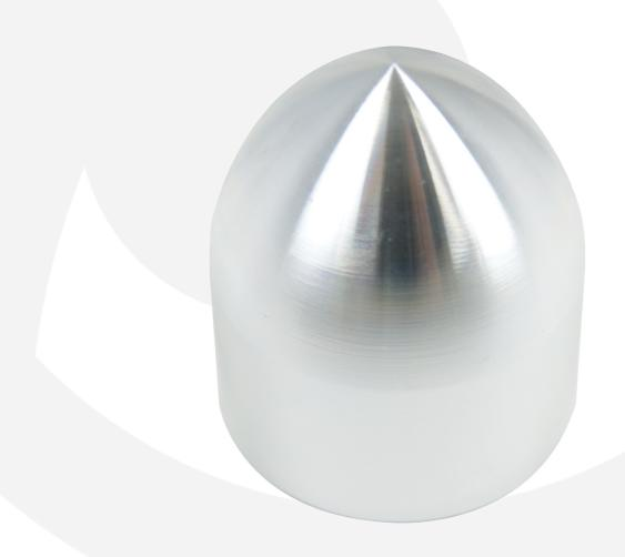
The aluminium phase plug is designed to replace the standard plastic one on the SPL8M.1. When installed, this accessory increases power handling noticably as it dissipates the heat much more effectively than the standard plastic unit.
