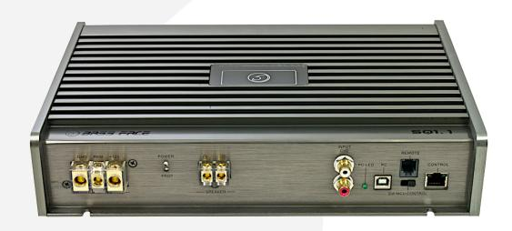
Time to lay on some power. Connect the earth first, then 12V power, then remote. Then connect in the RCA cables and you can move onto setting up sound controls on the amplifier. This description covers the principles of operation – for specific instructions refer to the set up notes for the exact model you are working with.
