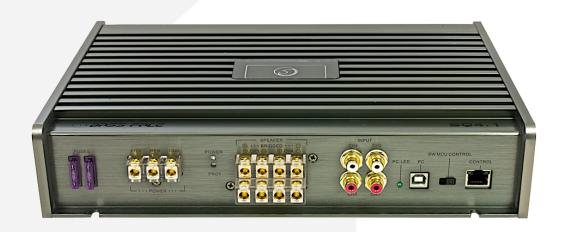
Time to lay on some power. Connect the earth first, then 12V power, then remote. Then connect in the RCA cables and you can move onto setting up sound controls on the amplifier. This description covers the principles of operation – for specific instructions refer to the set up notes for the exact model you are working with.
